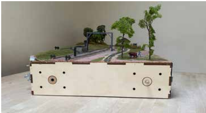
Wooden dowels are useful to get horizontal and vertical positions correct
