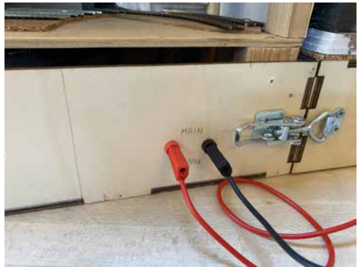
Banana plugs provide electrical continuity
