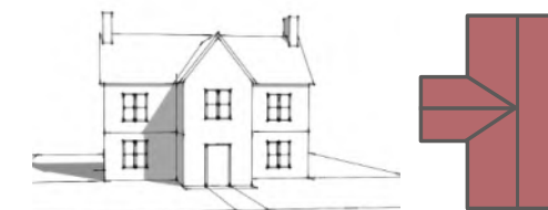
Traditional farmhouses are another example of ‘T’ shaped buildings. Attention should be paid to symmetry and proportions
