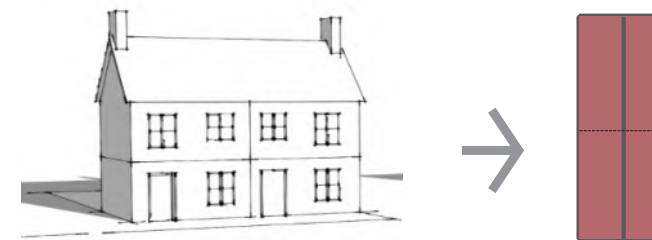
Simple cottage designs are predominant. A typical span is rarely greater than 6.5m in width, and usually around 5m.
