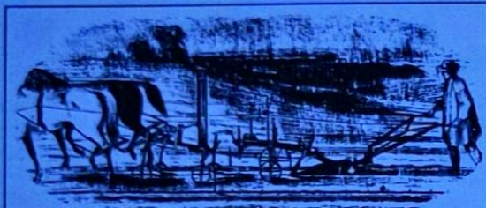
The Bentall Dynamometer attached to a plough to ascertain the amount of draught or labour performed by the horses in turning over the soil. It could also be used for any other purpose of a similar nature.
