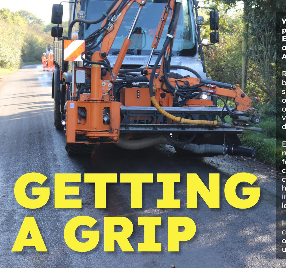
With Winter coming up and the probability of worsening weather, Essex Highways has been trialling a new Grip cutting Vehicle in Ardleigh, near Colchester.
