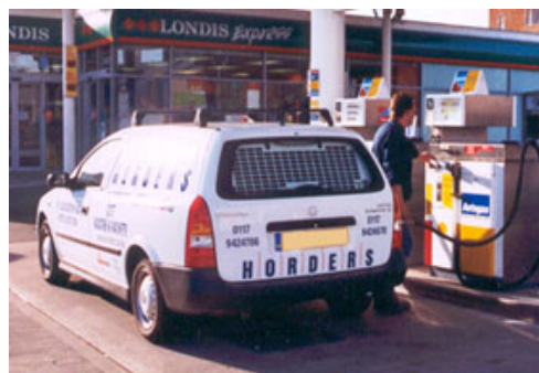
Figure 6.3 Vauxhall Astra 'Dual-Fuel' LPG car-derived van refuelling
