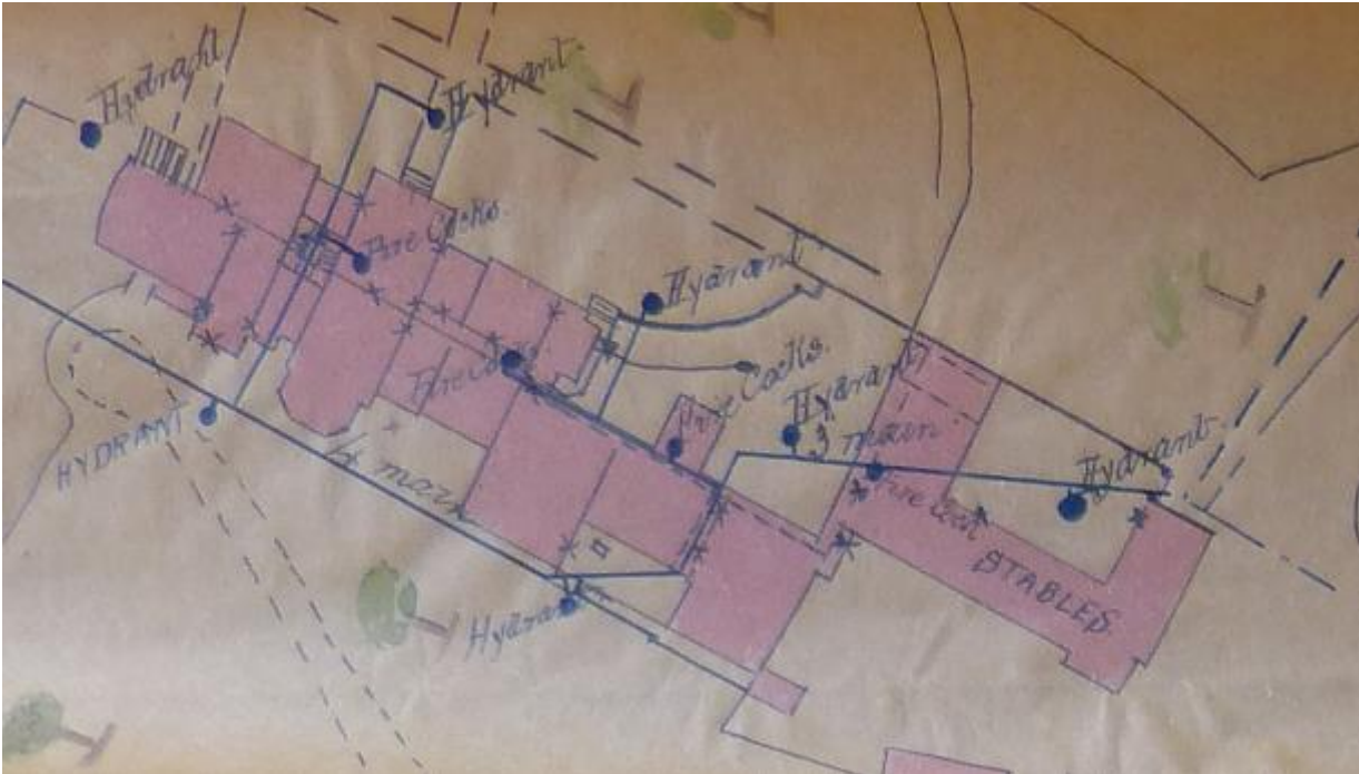
Plan of hydrants and firecocks:
