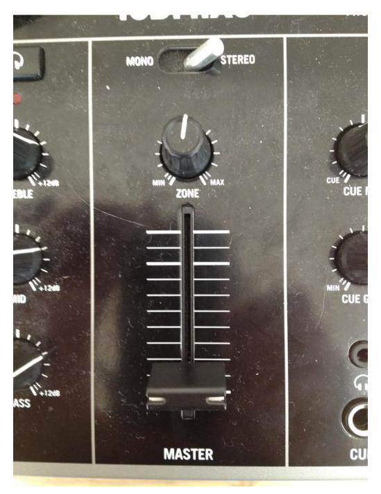
This slider is located within the middle of the main play deck. This slider controls the main system volume of all inputs, CD's, Ipods & the microphone.
