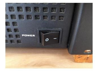
Amplifier Power switch, this is on the front lower of the PA system.
