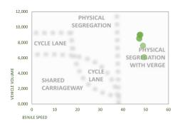
The cycle provision diagram compares total daily traffic flow (vertical axis) against the average daily 85%ile speed (horizontal axis) to demonstrate cyclist and vulnerable user considerations
