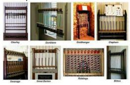
The more modern frames have "ratchet and pawl" sets that are used to winch the ropes to the required tension prior to chiming and which can be easily released after chiming has finished. However, some have only a set of hooks to fasten and unfasten individual ropes.
