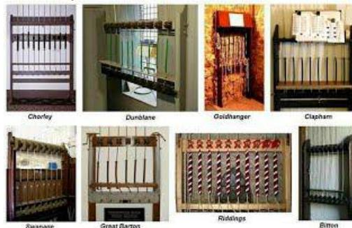
The more modern frames have “ratchet and pawl” sets that are used to winch the ropes to the required tension prior to chiming and which can be easily released after chiming has finished. However, some have only a set of hooks to fasten and unfasten individual ropes.
