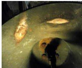
This photograph shows two polished area of wear on the inside of a typical bell caused by the chimes hammer (on the left) and the clapper (on the right), resulting from 50 to 100 hundred years of use. The extended diagonal area caused by the chimes hammer shows that it has occasionally struck the bell very close to the rim.
