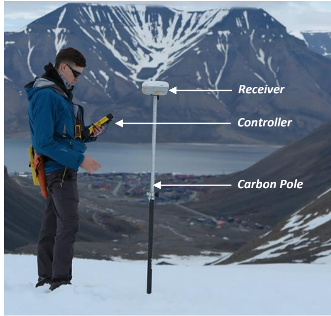
Figure 4.1: Trimble R4 Rover DGPS setup
