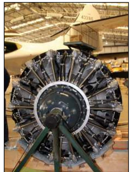
Our lovely new engine fresh back from the workshops of Anderson Aeromotive in Idaho and ready for hoisting aloft to be mated to the engine mounts on the port wing
