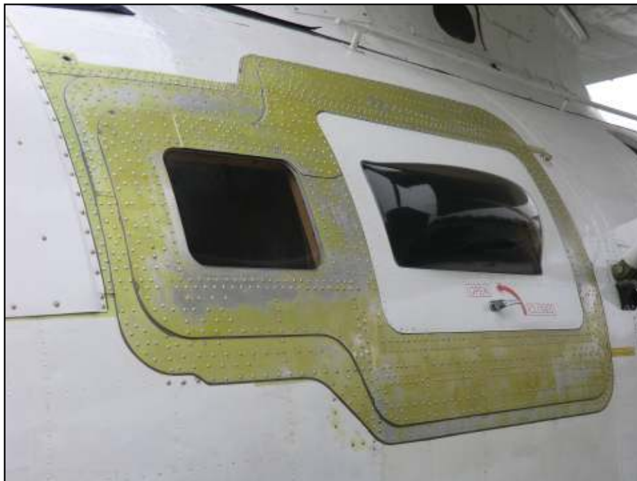
A close-up of the work that has been carried out by engineer Garry Short on the port side forward hull of Miss Pick Up at Duxford this winter. The new window is to the left and it can be seen that the whole area has been 'beefed-up' structurally. In due course, the metalwork will be painted white to match the rest of the hull David Legg
