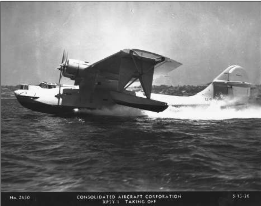
The prototype XP3Y-1 flying boat that led to the famous PBV line, here seen on May 15 th 1936 taking off from the sea near San Diego, California David Legg collection
